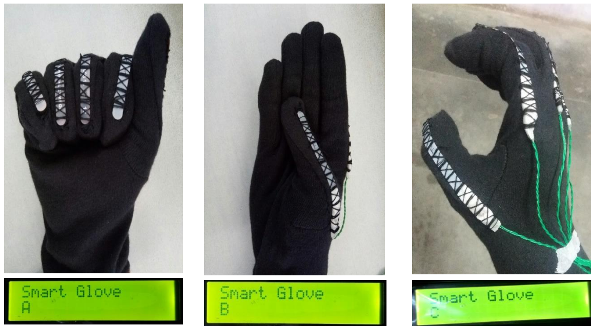
Fig. 5: Hand Gesture being converted to text using the proposed design
