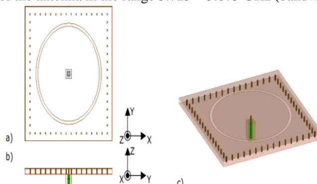
Fig. 5 Structure of single planar antenna with circular slot (in scale 1:1): a) top view; b) side view; c) 3-D view
