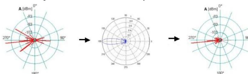
Fig. 9 Elimination of some multipath components using narrow beam antenna in the receiver
