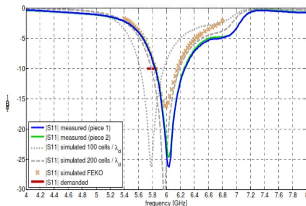
Fig. 7 Measured and simulated reflection coefficient the antenna.
