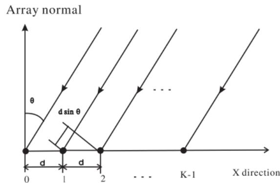
Fig. 1 Antenna array representation.
