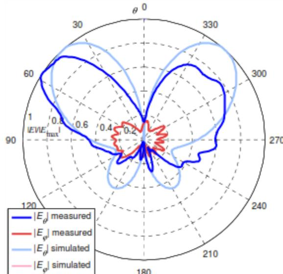
Fig. 8 Measured and simulated XZ-plane cross-section of radiation pattern
