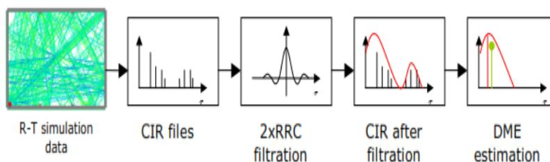
Fig. 11 CIR generation and filtering process using DEES program
