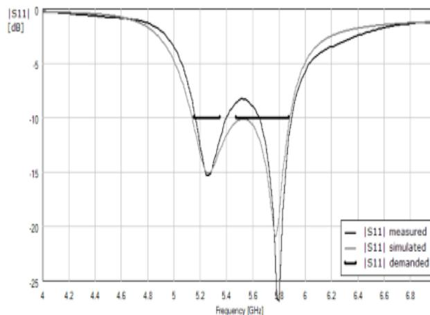
Fig. 4 Reflection coefficient of the antenna
