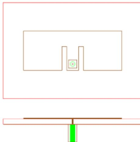
Fig. 2 Structure of E-shaped patch antenna, top view and side view.
