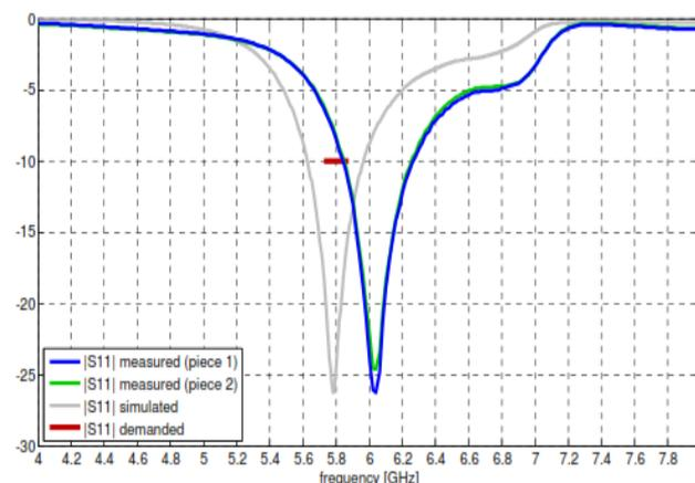
Fig. 6 Measured reflection coefficient of the antenna
